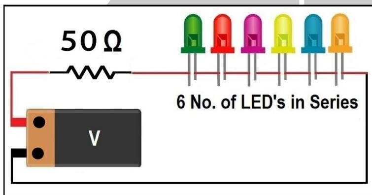
**Note: LEDs are of 1.3V, 10 mA rating. There can be relevant changes in this.**
